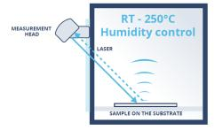
CurinScan is based on Nanoscale Mobility Analysis (NMA) and measures the structure (particles, polymers, pigments...) Brownian motion. During the film formation or curing process, structure nanoscale mobility changes due to the change in the material properties, for example from liquid to solide. The insitu analysis of the nanoscale mobility provides a full reading of the thermodynamic mechanisms and characteristic times.
