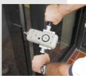
The DMG ergonomic gauge lets you objectively measure manual muscle strength and functional task requirements for almost any application.
