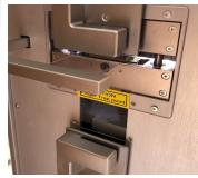
Two sample clamps above and below the Film Feeding Blade are used to hold the sample. In manual loading mode the user controls the clamps and loads a single sample. In automatic mode, the sample clamps are controlled by the PLC after initial loading on to a spool.
