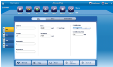
Digital test methods include; Sample ID, Material ID, Film/Package mode, material thickness, & Conditioning Time
