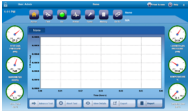
The Home screen shows the Carrier and Test Gas pressures, barometer, and block temperature.
