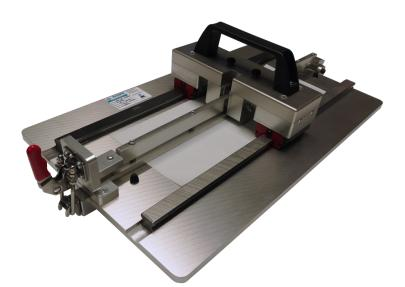
The cutter has two blades mounted to a separate holder and therefore can be replaced easily when blunt. The blade holder is mounted onto a draw down carriage which is guided and running on two rails, this ensures parallel running and precise cutting. A film clamp holds the film tightly to assist in the cutting of the material.
