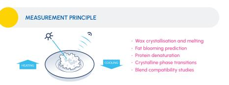
Rheolaser Crystal uses the Diffusing Wave Spectroscopy principle (DWS). Light is scattered by the particles, creating an interference pattern (Speckle Image). The variation of this image is directly related to the motion of the particles: the faster they move, the faster the Speckle Image changes. By a mathematical analysis of this variation, decorrelation functions can be computed and then processed, to obtain a characteristic time [], as a function of time or temperature.
